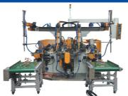
Chipless cutting & bending & end forming integrated machi (one set cutting device and two sets of separate bending de
