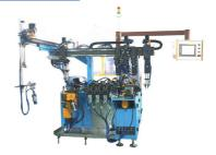
Chipless cutting & bending & end forming integrated (one set cutting and bending device only)
